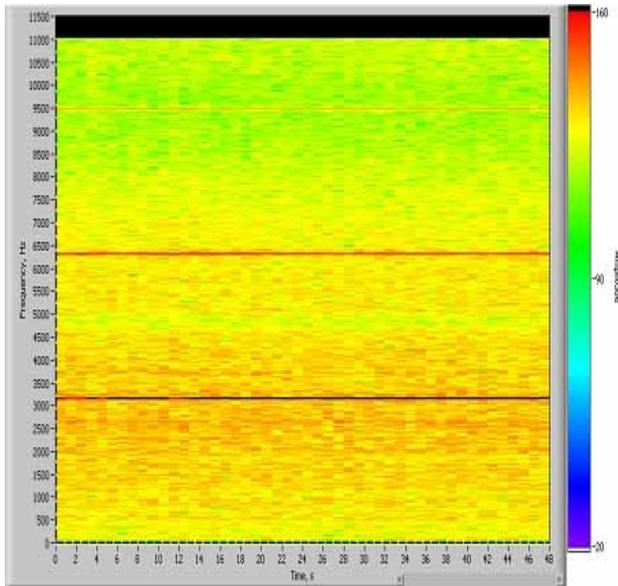
**Fig. 6** The audio spectrum, obtained from the vortex chamber (Fig. 1,  $d = 30$  mm,  $P = 5$  bar).
