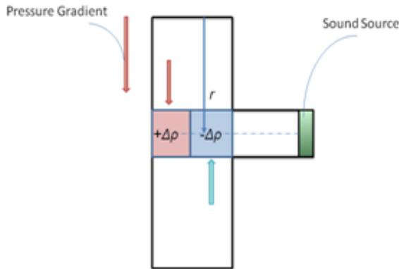
Fig. 8 Volume filled with a gas inside a field of forces, creating pressure gradient.
