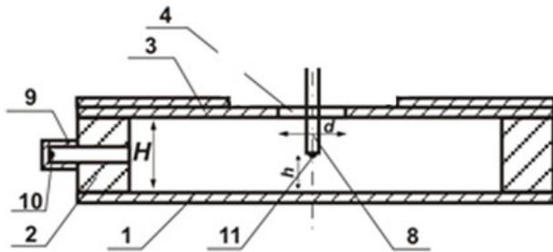
Fig. 3 Schematic overview of modified experimental vortex chamber (cross-section front view). 1—lower disc; 2—cylindrical side wall; 3—upper disc; 4—outlet diaphragm; 8—central rod; 9—plugged branch pipe; 10—“hot” thermocouple; 11—“Cold” thermocouple;  $H$ —vortex chamber height (25 mm);  $d$ —outlet diaphragm diameter;  $h$ —distance between central rod and lower disc.
