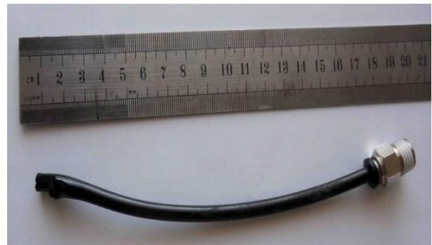
Fig. 5 The broken piece of polyethylene tube.
