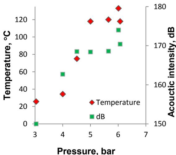
**Fig. 7** The heating of “hot” thermocouple and acoustic intensity as functions of inlet pressure.
