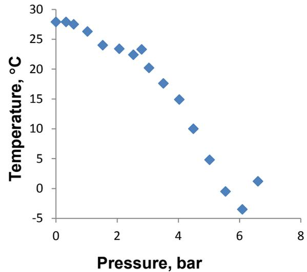
Fig. 4 The temperature measured by “cold” thermocouple (Fig. 3) as function of inlet pressure.
