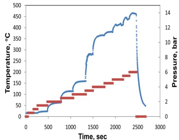
**Fig. 2** The experimental file of the vortex chamber with outlet diaphragm  $d = 30$  mm. The readings of inlet pressure and temperature ("hot" thermocouple) were recorded every second.
