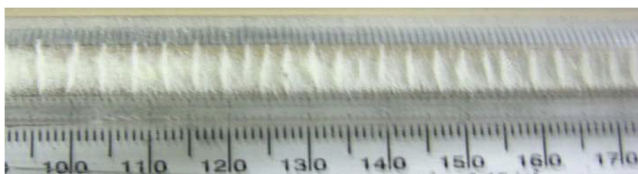
Fig. 3. Photo of periodic structure inside the transparent cavity of Hartmann sound generator.
