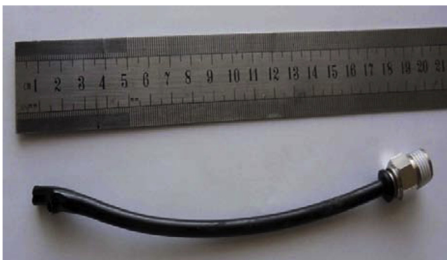
Fig. 5. The broken piece of polyethylene tube.
